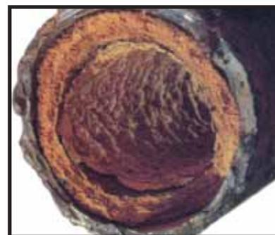
*Boiler scale building up on the inside of a lead water pipe. If hard water passes through water pipes, the inside of the pipe is covered with  $\text{CaCO}_3$ ,  $\text{CaSO}_4$  and  $\text{MgCO}_3$ . Therefore, lead can not be used in water pipes, thus preventing the transfer of poisonous  $\text{Pb}^{+2}$  ions to the water.*
