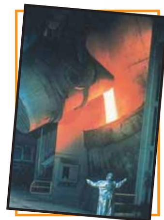
A molten iron charge is added to a basic oxygen furnace.
